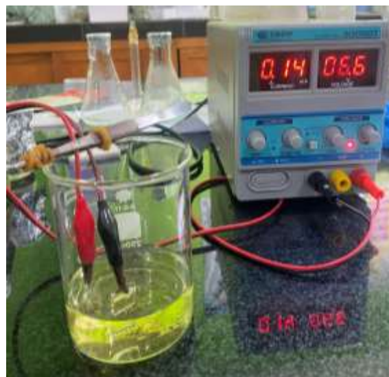
Figure 1. Schematic of FTO Glass Coating with Pt
