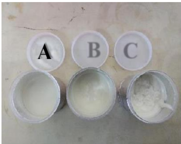
Figure 1. Sunscreen cream containing the active ingredient suji leaf ethanol extract encapsulated in the nanoparticle system A:FI (T80:SA (3:3)% w/v), B:FII (T80:SA (3:10)% b/v), C:FIII (T80:SA (10:10)% b/v).
