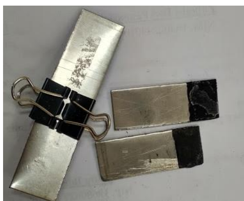
Figure 4. Cocoa skin supercapacitor electrode.
