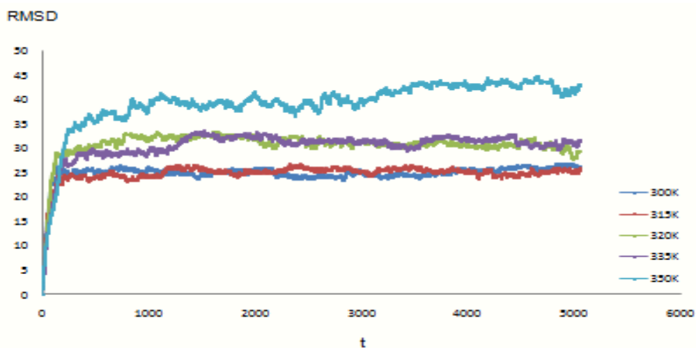
Figure 4. RMSD curves (Å) at 300 K, 315 K, 320 K, 335 K and 350 K versus the simulation time (t).
