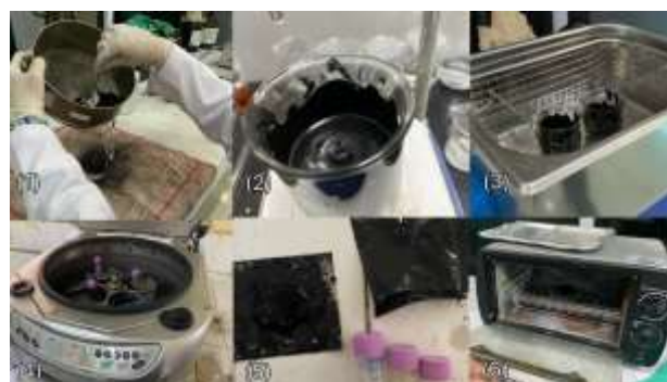
Figure 3. The synthesis process includes: sieving (1); dissolving and stirring (2); sonication (3); centrifugation (4); centrifuged sediment (5); drying graphene to powder (6).
