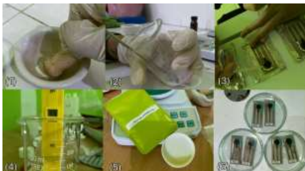
Figure 5. AgCl particle reduction(1); AgCl paste preparation(2); drop-casting of reference electrode(3); enzyme solvent buffer pH 5.5(4); glucose oxidase enzyme(5); enzyme incubation(6).
