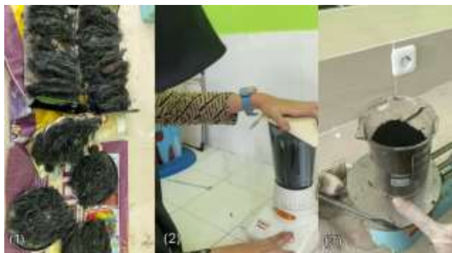
Figure 2. Combustion results using oven (1); charcoal crushing process (2); EOPB charcoal powder (3).
